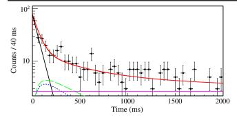
FIG. 2 (color online). Time distribution of the  $\beta$ -decay events correlated with implanted <sup>79</sup>Ni. The fitting function (solid red line) considers the activities of parent nuclei (dashed-dotted black line),  $\beta$ -decay daughter nuclei (fine-dashed blue line),  $\beta n$ -decay daughter nuclei (dashed green line), a constant background (solid pink line), and other decay products (granddaughter nuclei, etc.), which are not drawn in the figure.
