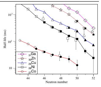
FIG. 3 (color online). Experimental half-lives as a function of neutron number for the isotopes with Z = 27-31. All the solid symbols represent the half-lives determined by this work while the open symbols are the half-lives taken from Refs. [21,23,24,35]. The systematic trends in different isotopic chains are highlighted by lines connecting the data points with a smaller uncertainty.
