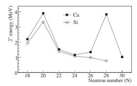
FIG. 3. Energies of the  $2^+$  states measured in the Ca and Si isotopes. Present result for  $^{40,42}$ Si—770(19) keV—brings evidence for the collapse of the N=28 shell closure at Z=14.
