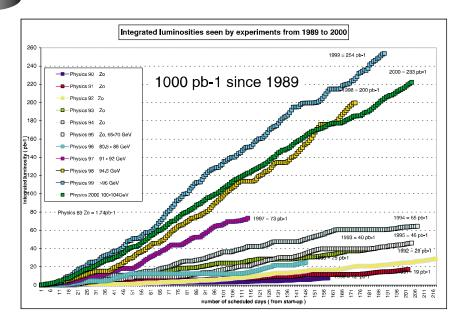
The luminosity delivered over the years of LEP running. The machine was pushed to deliver the highest possible beam energies while continuing to deliver high luminosity. The Z lineshape and W mass measurements rely on a precise calibration of the LEP beam energy, taking into account systematic effects including Earth Tides and leakage of electric current from nearby railway lines.
