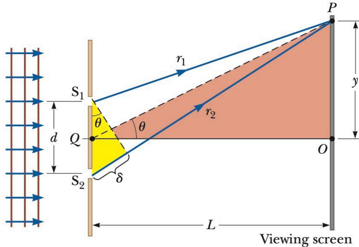
In the double slit experiment, supposed  $d = 0.100$  mm and  $L = 1.00$  m, and the incident light is monochromatic with a wavelength 500 nm.
