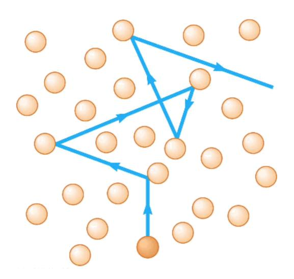
The mean free path, of a molecule is the average distance that a molecule travels before colliding with another molecule. It is given by
