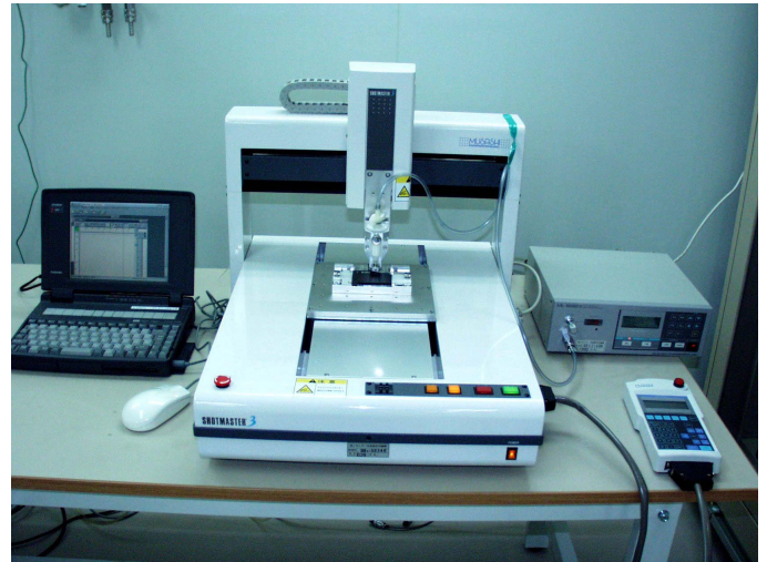
Figure 11: Glue dispensing system which is made of (1) a xyz stage where the baseboard is on the xy stage and a glue-syringe is attached on the z-axis, and (2) a dispensing controller.
