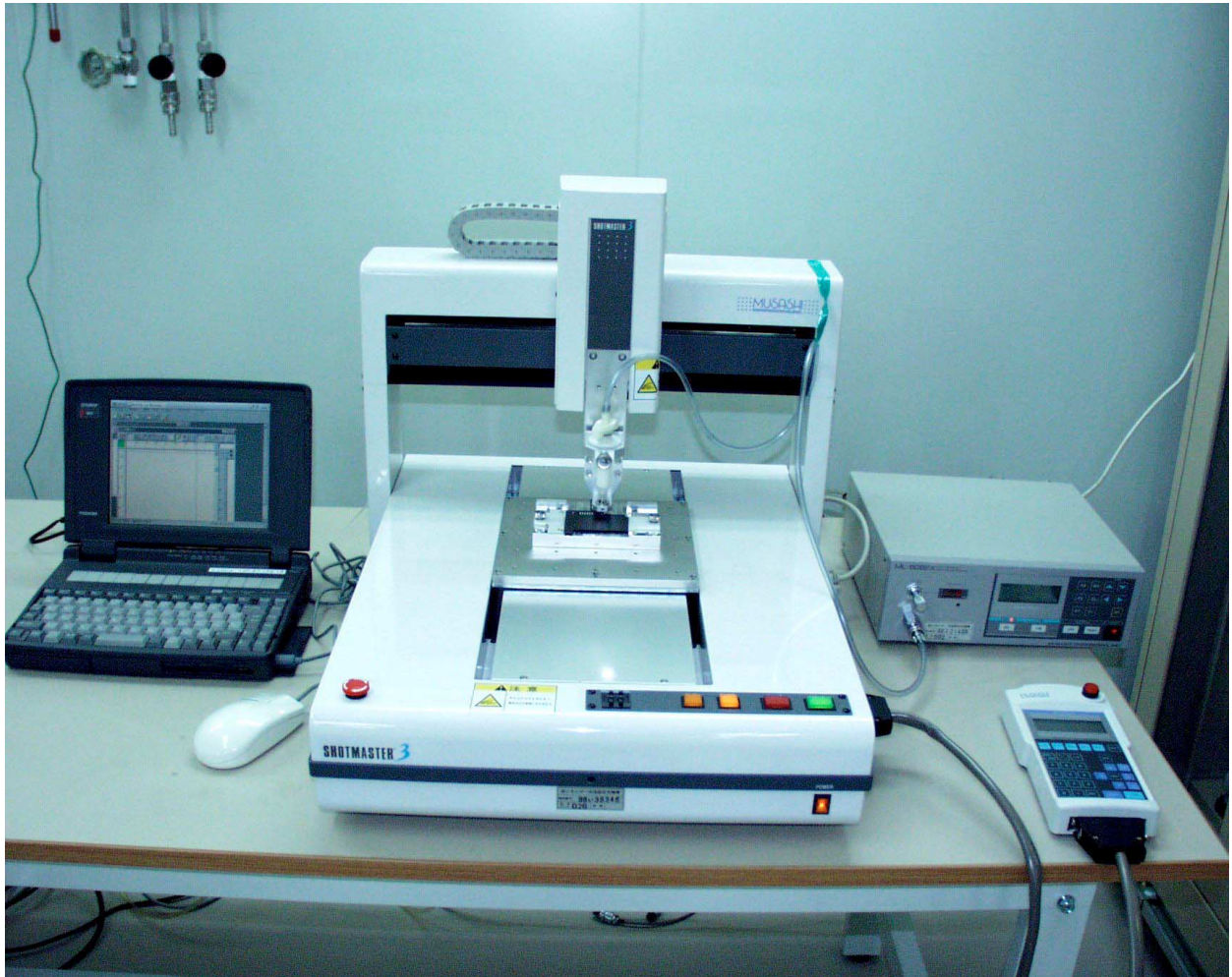
Figure 2 Glue dispensing system which is made of (1) a xyz stage where the baseboard is on the xy stage and a glue-syringe is attached on the z-axis, and (2) a dispensing controller.
