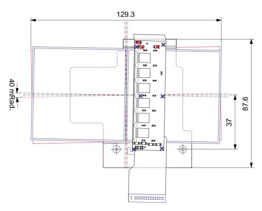
Figure 4 Survey of surfaces of hybrid and of large capacitors in the far-end. The surface of the hybrid is measured in open space at six locations: two in the near-end, two in the middle, and two in the far-end.
