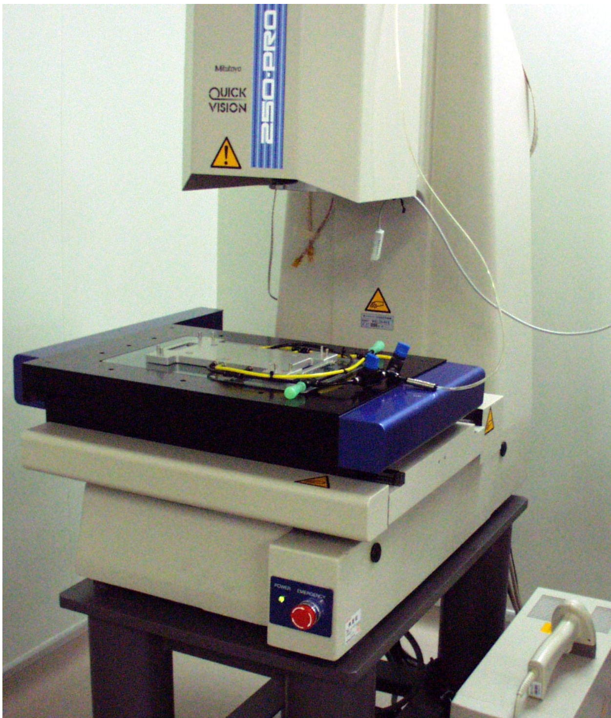
A base plate is placed on the measuring table of Quick Vision Pro250
