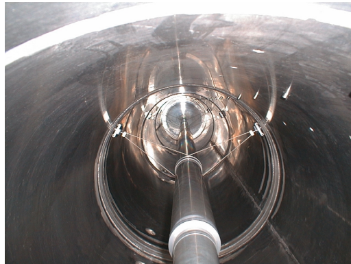
View inside the horn - "spider" support of inner conductor
